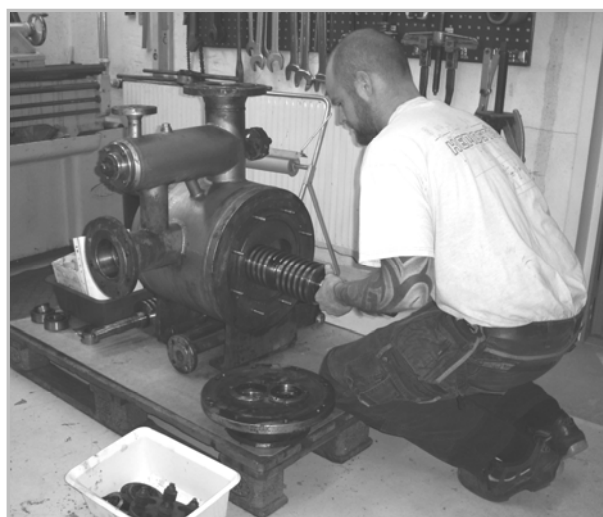
Bornemann W5.2zk-20 under reparation
