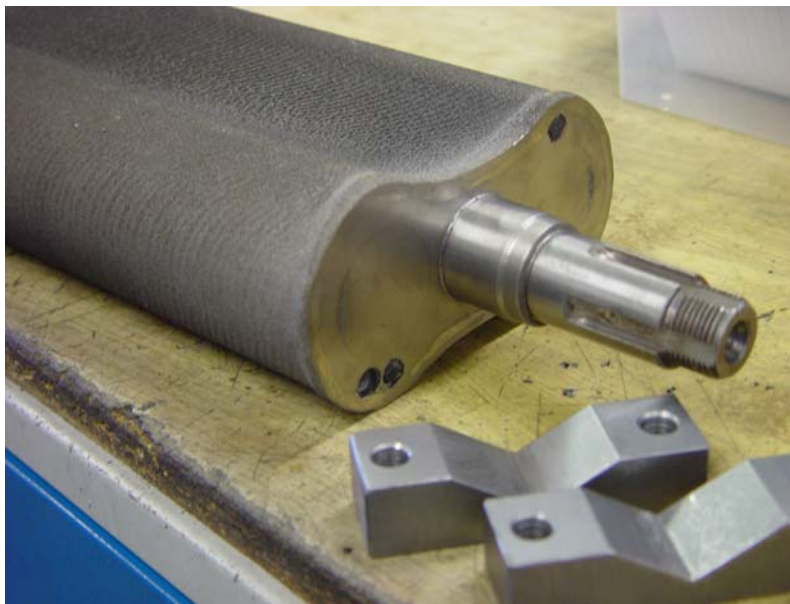
Rotor with protection layer AISI 316L prior final machining
