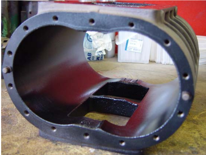
Finished casing with PTFE sealing layer over AISI 316L
