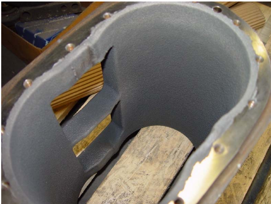
Protection layer in place before machining
